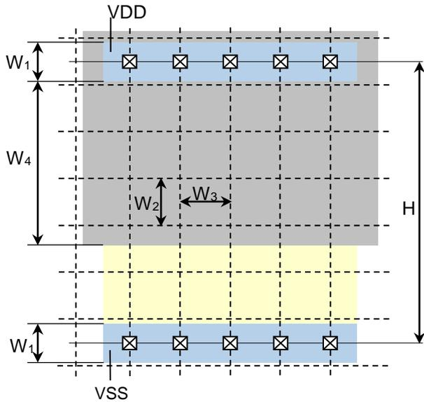
Fig. 6. Physical structure of single height cells
