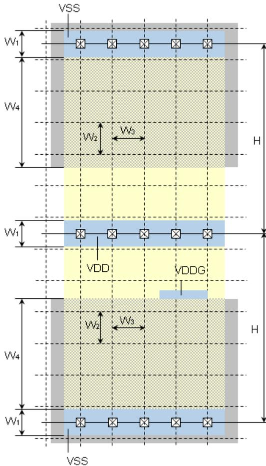
Fig. 7. Physical structure of double height cells
