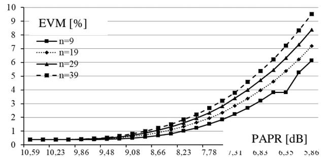
Fig. 7. The EVM of WCDMA signal at the PW filter output as a function of PAPR. The filter order values are: N=9, 19, 29, 39
