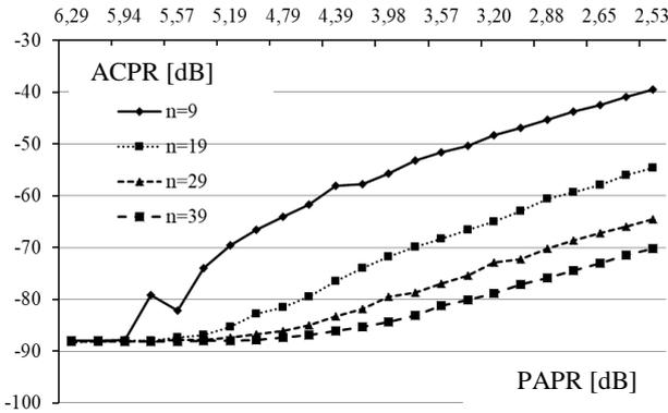
Fig. 4. The ACPR for QPSK signal at the PW filter output as a function of PAPR. The filter order values are: N=9, 19, 29 and 39
