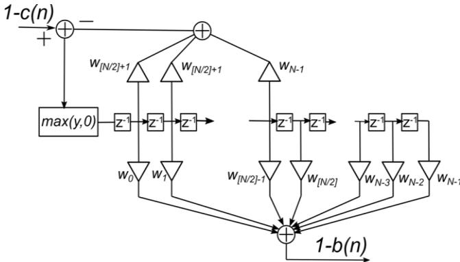
Fig. 2. The Peak Windowing CFR filter architecture
