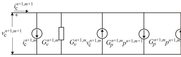
Fig. 1. The linearized and discretized model of the capacitor controlled by pressure
