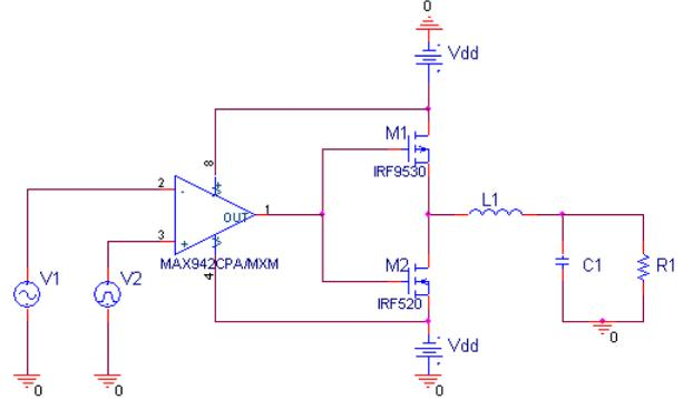
Fig. 4. The PSpice scheme of class-D PWM amplifier
