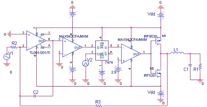
Fig. 5. The PSpice scheme of class-D PDM amplifier
