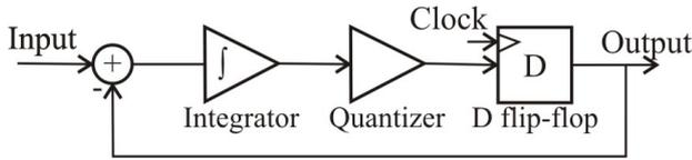
Fig. 3. First-order sigma delta ( $\Sigma\Delta$ ) modulator
