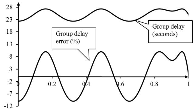
Figure 7. 9<sup>th</sup> order LSM filter with 6<sup>th</sup> order corrector. Group delay (up) and error in approximation of constant group delay (down)
