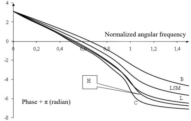
Figure 3. Phase characteristics of the 7<sup>th</sup> order CMAC and Chebyshev filters
