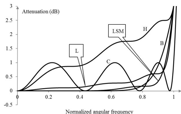
Figure 1. Attenuation characteristics of 7<sup>th</sup> order CMAC filters, and attenuation characteristics of Chebyshev filter with 1dB attenuation in the pass-band
