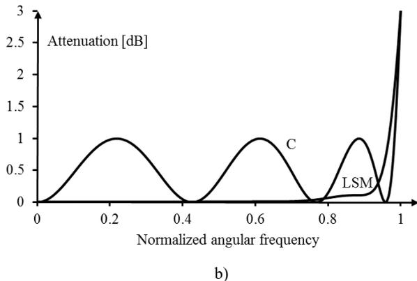
Figure 5. a) Attenuation in the stop-band and b) Attenuation in the pass-band of 7<sup>th</sup> order Chebyshev filter (1 dB, renormalized) and of 9<sup>th</sup> order LSM filter
