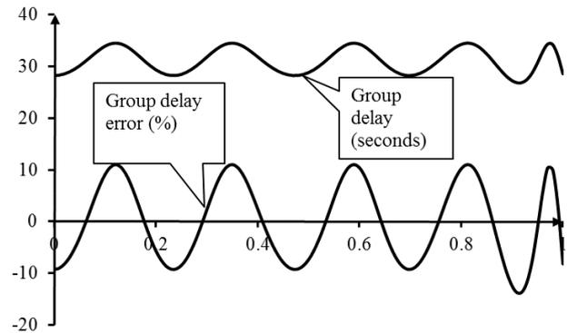
Figure 6. 7<sup>th</sup> order Chebyshev filter with 8<sup>th</sup> order corrector. Group delay (up) and error in approximation of constant group delay (down)
