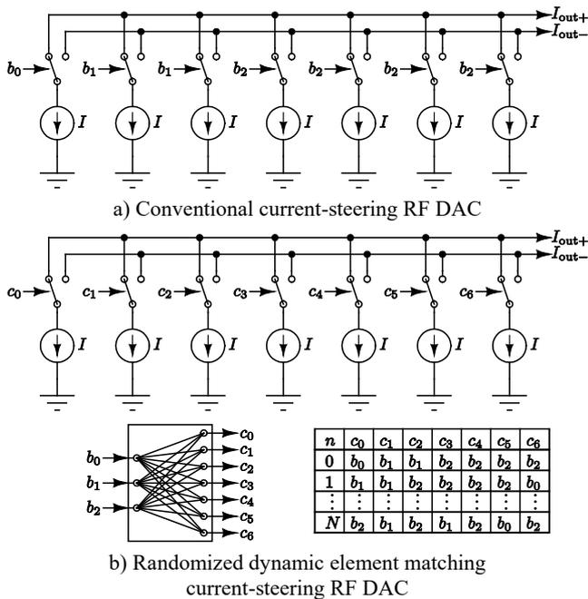
Fig. 4. Conventional and RDEM current-steering RF DACs
