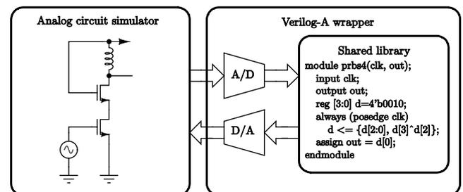
Fig. 2. Proposed solution for periodic steady state mixed-signal simulation
