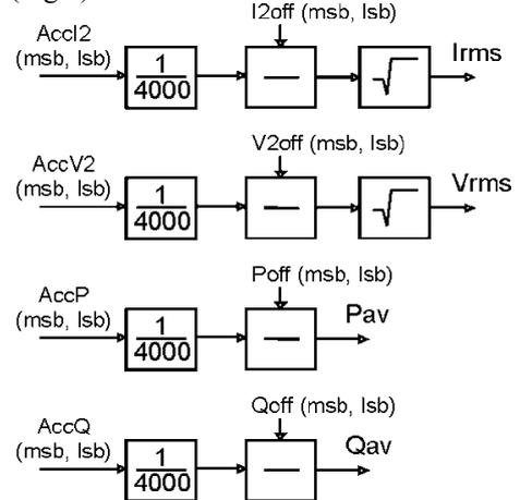
Fig. 5. The calculation of  $I_{RMS}$ ,  $V_{RMS}$ ,  $P_{AV}$  and  $Q_{AV}$
