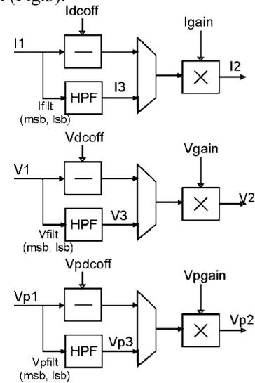
Fig. 3. The operations for DC offset eliminations
