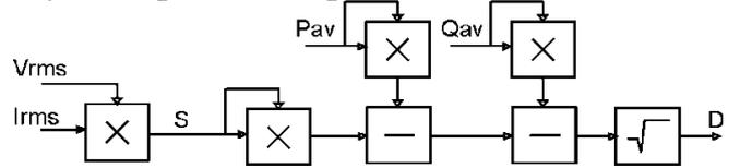
Fig. 6. The calculation of apparent power  $S$  and distortion  $D$
