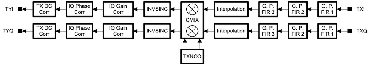
Figure 3: Structure of the TXTSP
