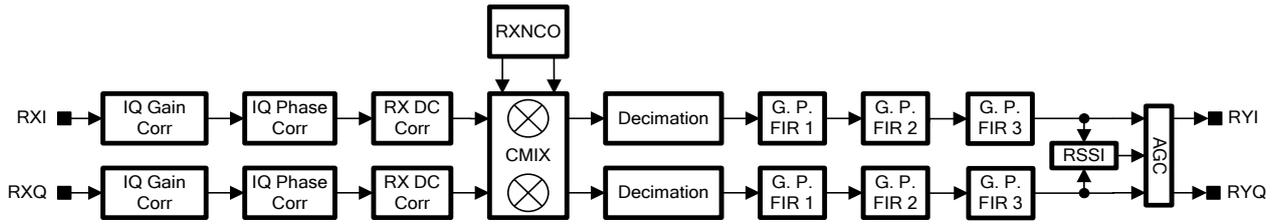
Figure 2: Structure of the RXTSP
