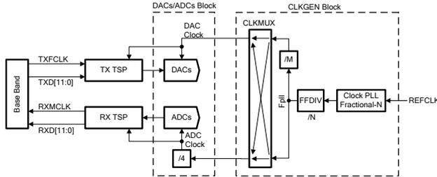
Figure 5: Clock generation and distribution
