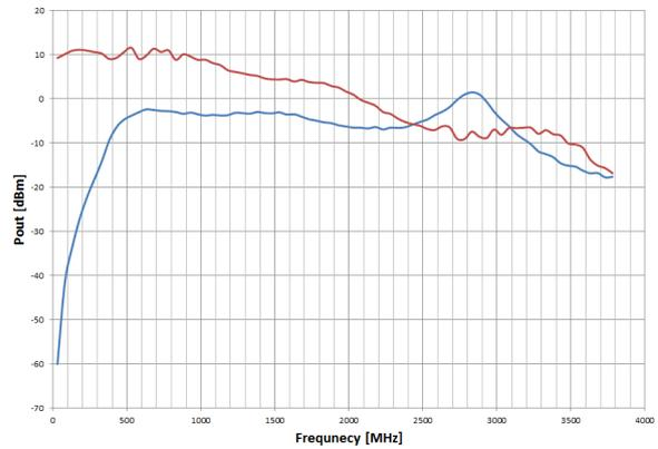
Figure 7: Transmitter gain versus frequency
