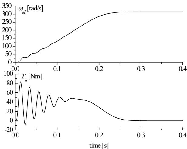
Fig.3. Speed and electric torque during free acceleration
