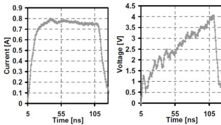
Fig. 4. Voltage and current chronograms of an interconnection for a TLP voltage pulse with a 100ns duration.
