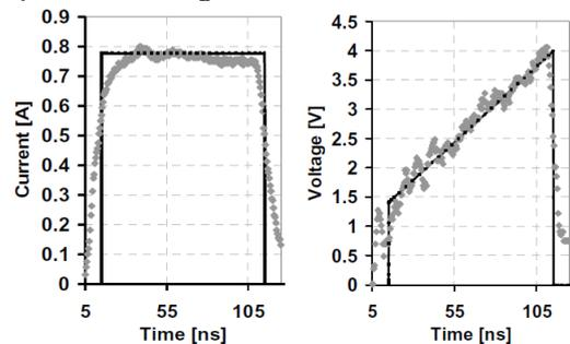
Fig. 8. Voltage and current chronograms of an Interconnections (TLP voltage pulse, 100ns duration)
