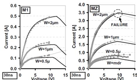
Fig. 10. VF-TLP IV curves of interconnections, 45nm technology: two metal layers M1 and MZ, measurements-Gray and simulations Black for 30 ns square pulses
