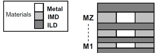
Fig. 1. Cross section of metal layers stacked
