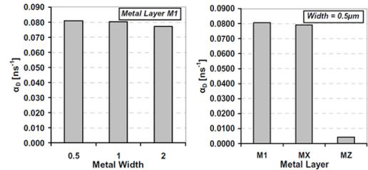
Fig. 7.  $\alpha D$  coefficient value for different widths of metal layers
